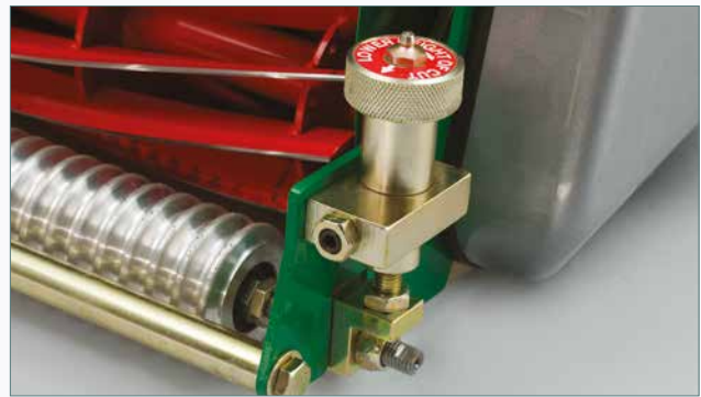
Positive, easy height of cut adjustment in 0.25mm increments
