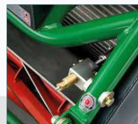
Easy adjustment of bottom blade to cylinder
