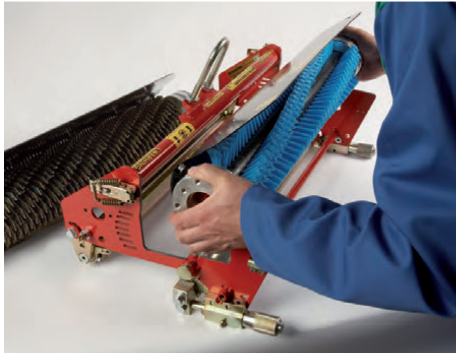
Simple, safe and secure cassette changeover.
