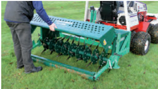
The hinged rear guard gives good access to the interchangeable attachments.
