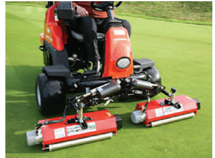
Select-A-Vibe rollers are available for both electric and hydraulic drive greens mowers.
