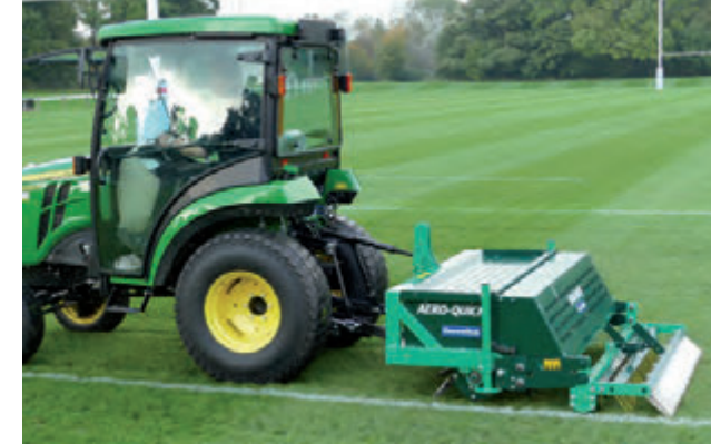
The Aero-Quick's 5' (1.5m) working width covers the track of most compact tractors and utility vehicles.
