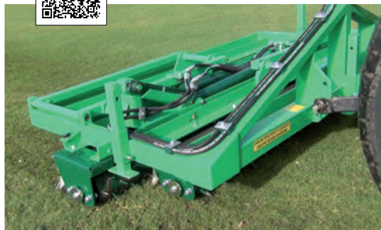
Units can also be used folded in for intensive overseeding preparation
